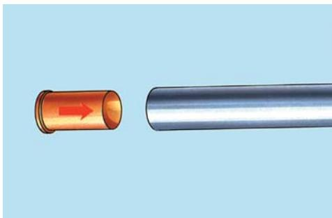
1. Check that the pipe end is free from scratches, burrs etc. Place supporting bush inside the pipe, if required.
