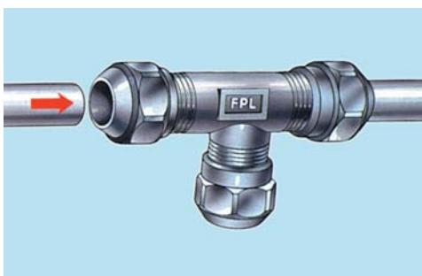
2. Push the pipe into the coupling as far as it will go, and hand tighten the thrust nut.
