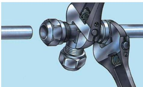
3. Tighten the thrust nut using a spanner: No of turns - see tabel. The cone is thus pressed firmly against the pipe, and forms a seal.
