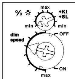
The minimum brightness (fully dimmed) is adjustable with the % ⚡ rotary switch.
